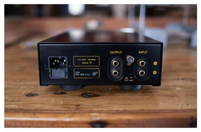
Two pair of single-ended RCAs take care of in and out connectivity with a grounding terminal between the input and output sides, while an IEC inlet completes the simple backside story.
